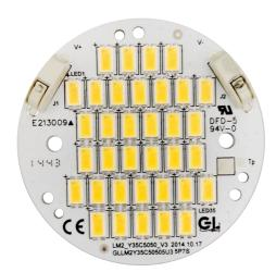
The maximum allowed temperature at the  $T_P$  point of the board is 80°C. This temperature is not based on the LM-80 standard but is for warranty purposes only.
